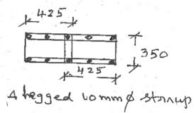
Provide four legged 10mm Φ stirrups @ 20mm c/c. Refer drawing.
